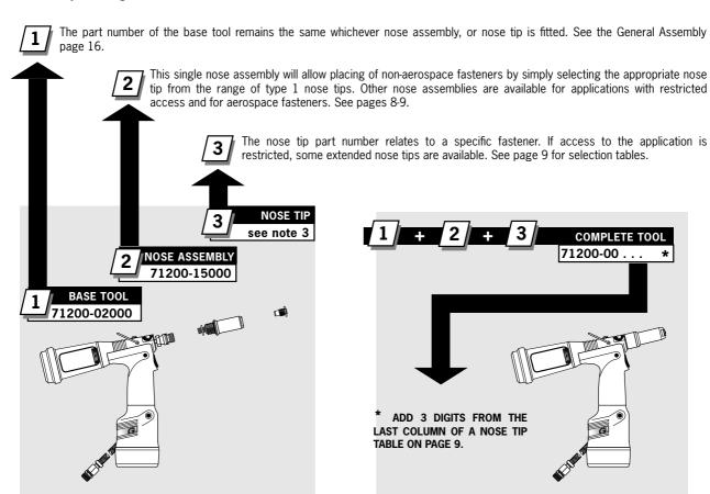
If you wish to place most of the fasteners in the table above, you can order the 71200-00039 complete tool comprising of:
