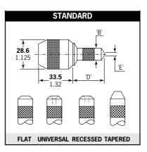
Available in 4 different end forms to place all fasteners (except Rivscrew). Suitable on applications with no or little access restriction.
