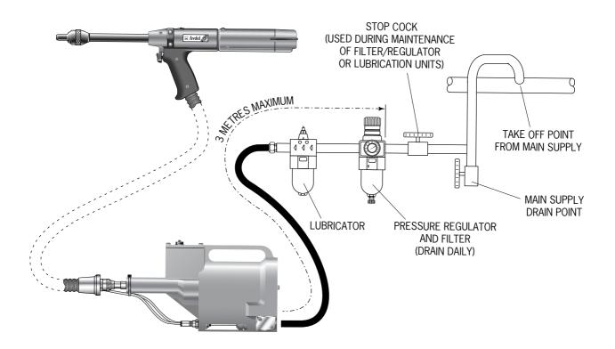
Follow the steps below when connecting the tool to the intensifier and main air supply:
